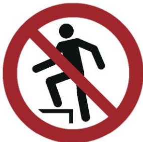
P019 Do not climb this area
