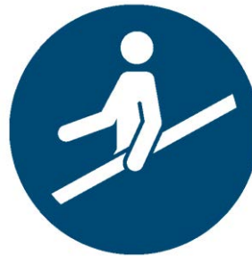
M012 Use handrail
