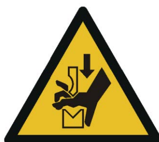
W030 Warning: Risk of squeezing hand between the tools of a press
