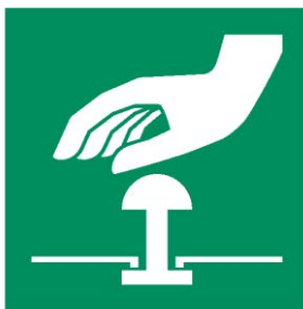
E020 Emergency shutdown button
