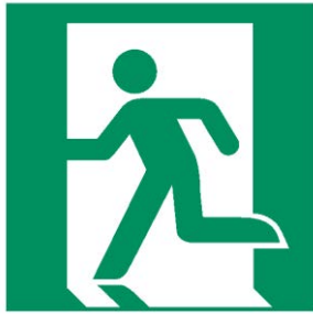
E001 Emergency exit (left)
