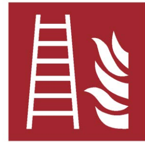
F003 Fire ladder
