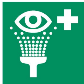
E011 Eye rinsing facility
