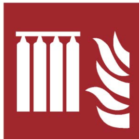
F008 F Stationary rack with fire-extinguishing agents
