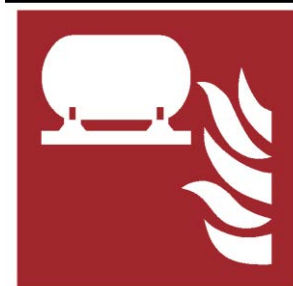
F012 Stationary fire-extinguishing system
