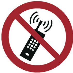
P013 No switched-on mobiles
